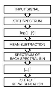
Fig. 1. Schematic structure of the MSA feature extraction.
