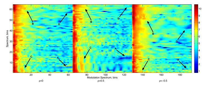
**Fig. 4**. Exemplar MSA feature set (log-variances of individual modulation spectrum bins through a speech sample). The plot is given for three values of  $\rho$ :  $\rho$ =0 (no distortion),  $\rho$ =0.5 (low spectral frequencies get stretched),  $\rho$ =-0.5 (high spectral frequencies get stretched). A, B, C, D - specific distinctive features on the spectral – modulation-spectral plane, which illustrate stretching and compression.
